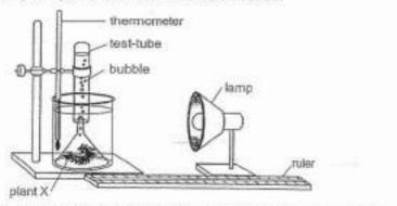
She switched on the lamp and counted the number of bubbles produced by plant X in one minute.
