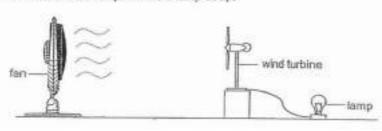
Meiling placed the wind turbine closer to the fan. She observed that the blades of the wind turbine spun faster and the lamp lit up more brightly.
