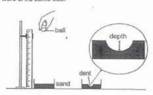
She dropped the balls from different heights onto a container of sand. She measured the depth of the circular dent created by each ball on the sand.
