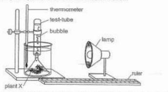
She switched on the lamp and counted the number of bubbles produced by plant X in one minute.
